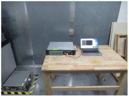
Asymmetric Mode Conducted Emissions(150kHz-30MHz)
